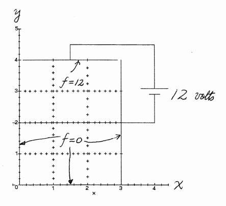
Given the boundary conditions as f(0,y)=0 , f(3,y)=0 , f(x,0)=0 and f(x,4)=12 volts ,
